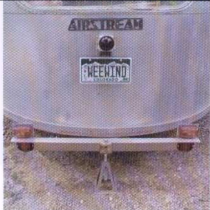
A temporary light bar gives Ruby modern safety while on the road, yet removes for vintage shows.
